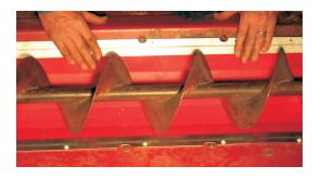
6. With the "Upper Rear" hold-down in place, install the "Upper Front Left" and "Upper Front Right" hold-down strips in a similar manner. NOTE: Take care to position the front strips parallel to the rear strip.
