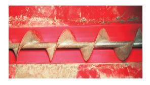
4. Insert one of the poly liners below the upper auger. Slide the liner to the left until it makes contact with the unloading auger housing, then center the liner between the bolt heads as shown.
