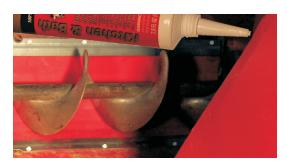
7. With both front and rear strips installed, reapply a silicone seal along the right end of the liner plus all three sides of the center brace.
